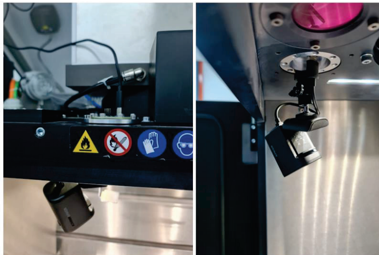
Figure 17: Anker PowerConf C200 Webcam is attached via a set screw on a modified port cover. A 15cm USB-C is used to connect the webcam to the customised PCB.
