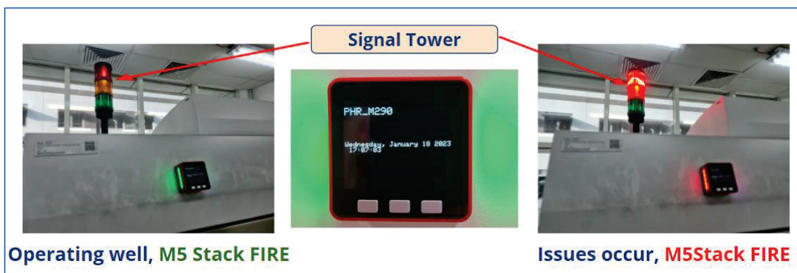
Figure 15: When the signal tower is not blinking, M5 Stack is lit green. When the signal tower flashes red light, the M5 Stack is lit red.
